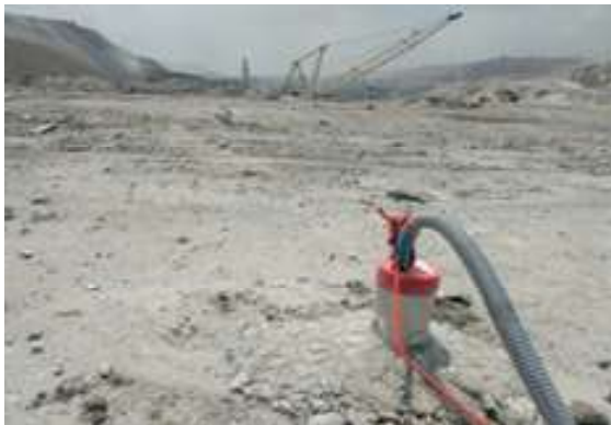
Fig. 5: Field placement of near-field sensor
