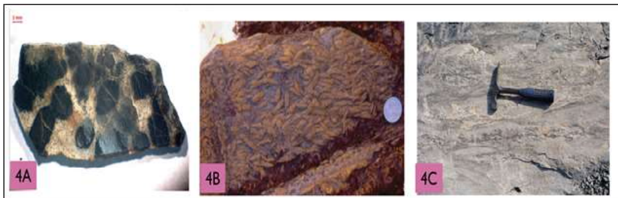
Figure 4: (4A) Cordierite dominated in hydrothermal alteration zones developed in felsic volcanic dominated volcano-sedimentary sequence at Deri Deposit; (4B): Pinnitized cordierite in hydrothermal alteration zones developed in felsic volcanic zone developed in volcano-sedimentary sequence of Deri Deposit; (4C): Cordierite forming greasy irregular patches in freshly exposed alteration zone in Open pit mine at Ambaji VMS deposit.
