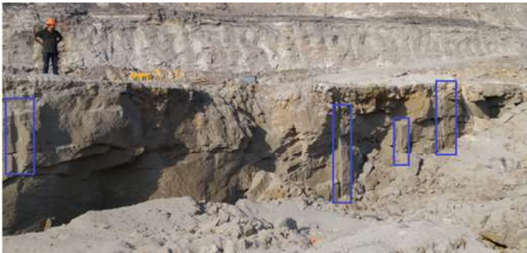
Fig. 9: Half cast impressions achieved in dragline bench
