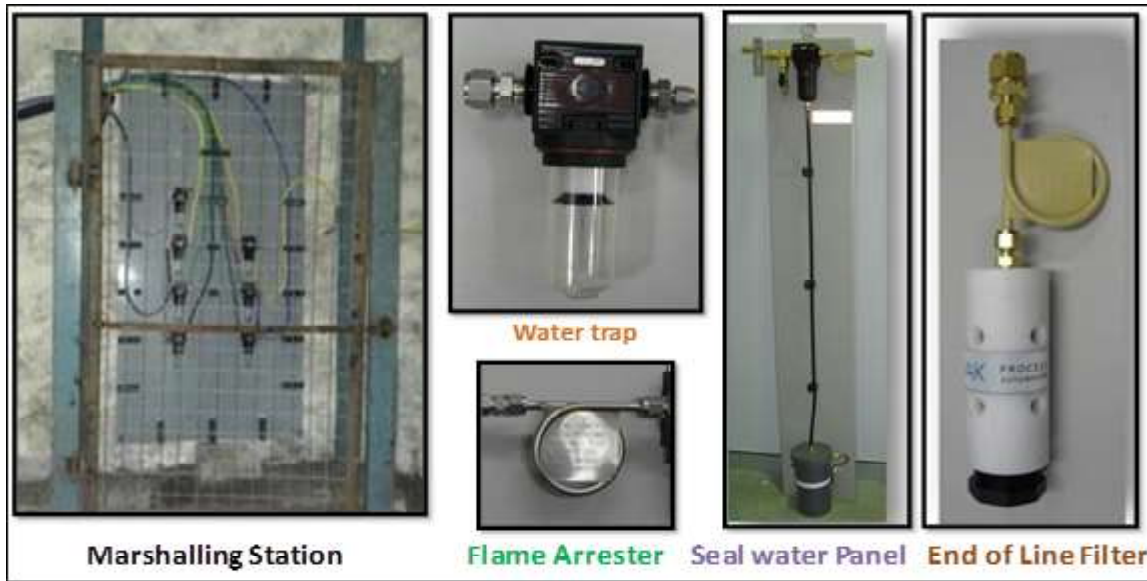
Fig.7: Marshalling station and the components of Tube bundle system
