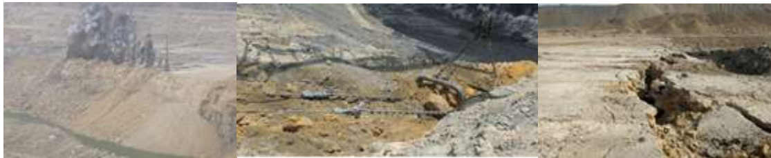
Fig. 1: Stemming ejection, poor fragmentation and backbreak in dragline bench blasting. This calls for advanced geo-engineering investigations for fine tuning the blasting system.
